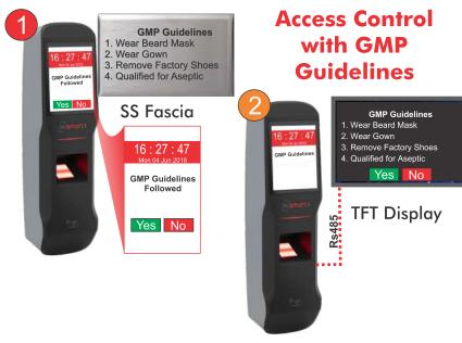
Enviro Technologies came up with access control solution with GMP prerequisites e.g. gowning, beard mask, factory shoes, gloves etc. which are mandatory to follow, failure of which will lead to no access in designated clean room or its peripheral area.
