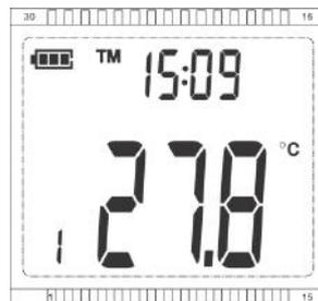
4. User can set DATE and TIME with pressing both 'SET' and "MIN/MAX" key at a time for maximum 5 sec. display will show 'S' symbol to indicate the device is in set mode. Display will show '00:' in time ("TM").
