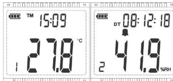
4. User can set DATE and TIME with pressing both 'SET' and "MIN/MAX' key at a time for maximum 5 sec. display will show 'S' symbol to indicate the device is in set mode. Display will show '00:' in time ('TM').
