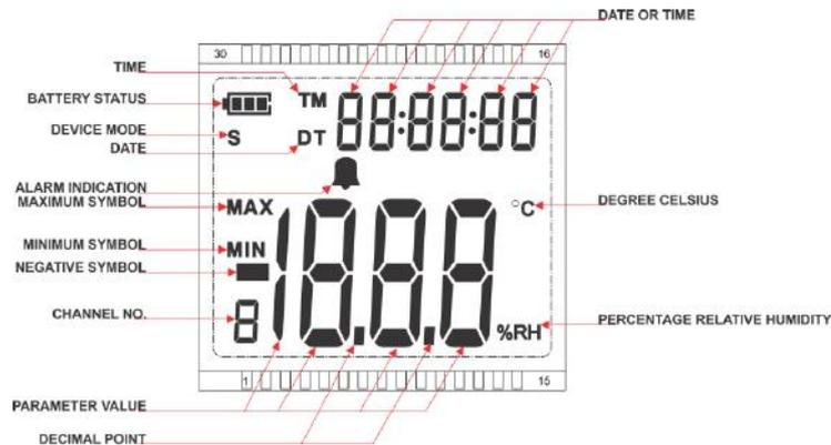
2. After inserting battery device will show information on display as below image.
