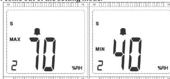
9. **Note :-** if we keep device in setting mode for more then 15-20 sec device will come out off the set mode. In this case device will save only new modified data up till it is modified, rest data will be as older value.
