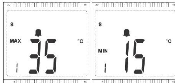
8. Further pressing 'MIN/MAX' key device will set humidity Maximum alarm setting. Using 'SET' key set humidity maximum alarm limit (0-99%RH no decimal value). Pressing 'MIN /MAX' key will set humidity minimum alarm limit (0-99%RH no decimal value). While setting alarm device will show bell symbol. Pressing 'MIN/MAX' key will save data in device and will come out of the setting mode.
