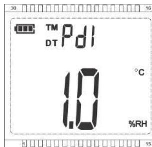
3. Power on device will start to show temperature and humidity reading. User can set date and time after replacing battery. Normally device shows data on display with temperature and humidity alternatively with 20 sec toggling time.
